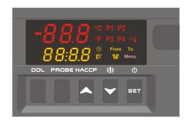
SET - Un programming mode it selects a parameter or confirm an operation. To start and stop recording, if the parameter rdb = y..
