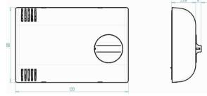
In order to censure a correct functioning the device has to be placed horizontally (as indicated by the figure above) so that the dIXEL logo can be read, only in this way the drilling on the case allow the correct inflow of air into the case.
