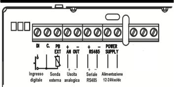
Here you can see the full wiring diagram. The presence/absence of analog output depends on the models.
