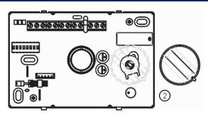
In case of box 503 installation, the cables should be arrive into the devices through the central hole as you can see as follow.
