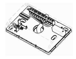
Otherwise, if need wireway so that you cannot use central hole. advised to make a small hole on the bottom of the case after havino removed the cover in order to avoid the possibility damage electronic board Please follow the figure nearby.
