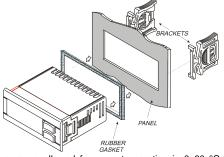
The temperature range allowed for correct operation is  $0\div60$  °C. Avoid places subject to strong vibrations, corrosive gases, excessive dirt or humidity. The same recommendations apply to probes. Let air circulate by the cooling holes.
