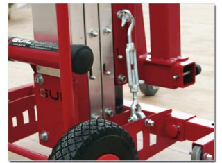
Adjustable mast blocking system for horizontal transportation.
