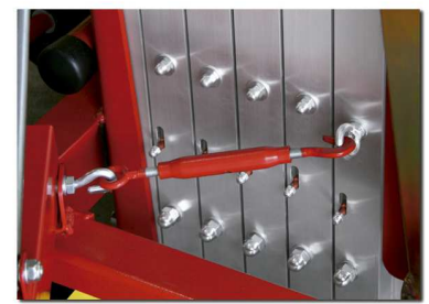
Adjustable mast blocking system for horizontal transportation.
