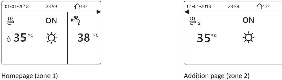
Figure 3-7.23: Set DOUBLE ZONE to YES and set ROOM TEMP. to NON; Set WATER FLOW TEMP. to YES or NON
