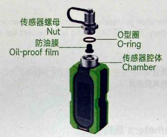
Oil-proof film is used inside of the vacuum chamber to filter impurities and reduce sensor contamination. To maintain optimal measurement accuracy, it is necessary to check the oil-proof film every three months for normal use (adjust the inspection cycle appropriately according to the frequency of use). If the oil-proof film is severely contaminated, it needs to be replaced.
