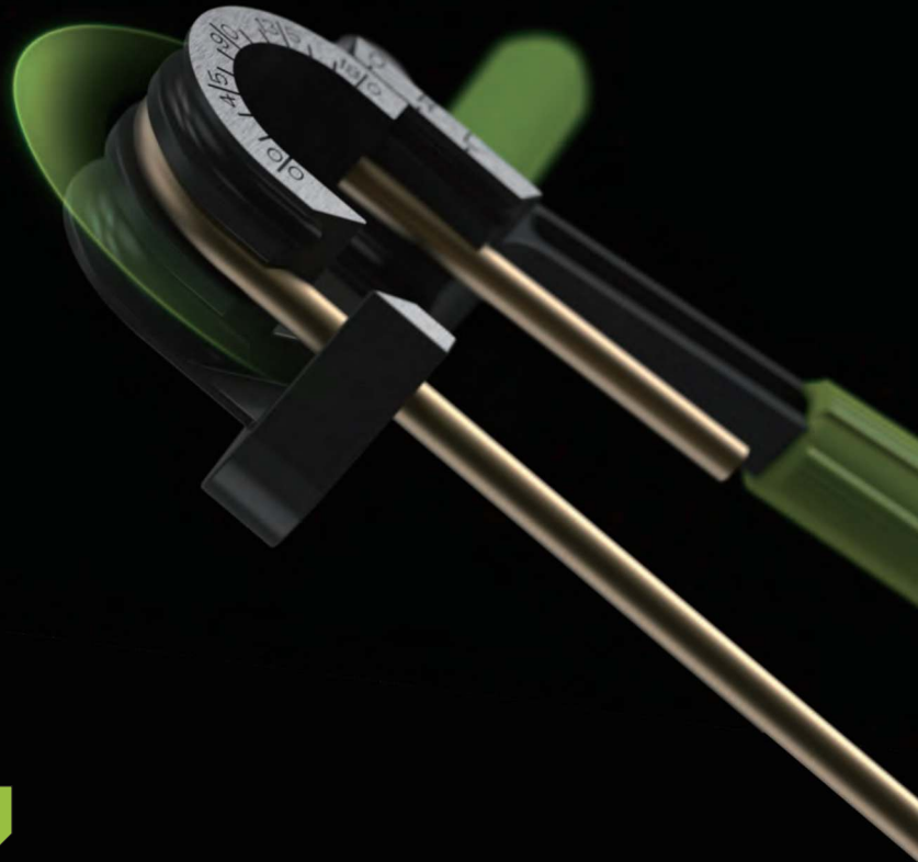
1 Please use a burner to heat a hard copper, then start the bending
